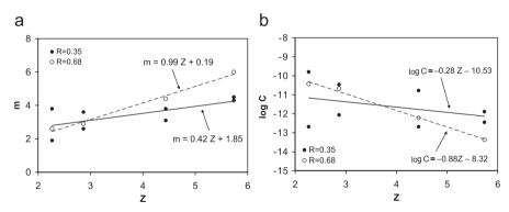
Fig. 7. The effect of R on the m-Z and  $\log C-Z$  relationships for tempered steels (experimental data from Evans et al., 1971, C evaluated using  $\Delta K$  in MPa  $\sqrt{m}$  and da/dN in m/cycle).
