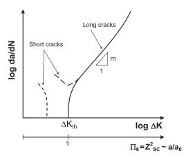
**Fig. 2.** Dependence of the crack growth rate on  $\Pi_6 = Z_{SC}^2$ .
