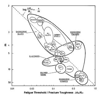
**Fig. 8.** Paris' law parameter m vs.  $\Delta K_{\rm th}/K_{\rm IC}$  (reprinted from Fleck et al., 1994 with permission).
