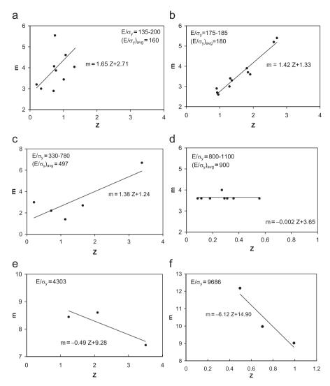
**Fig. 3.** Z-dependence of the Paris' law parameter m. (a) Aluminium alloys (Yarema and Ostash, 1975; Ostash et al., 1977). (b) 4340 steel (Heiser and Mortimer, 1972). (c) ASTM steels (Clark and Wessel, 1970). (d) Low carbon steel (Ritchie and Knott, 1974; Ritchie et al., 1975). (e) High strength concrete (data from Bažant and Shell, 1993 reinterpreted by Spagnoli, 2005). (f) Normal strength concrete (data from Bažant and Xu, 1991 reinterpreted by Spagnoli, 2005).
