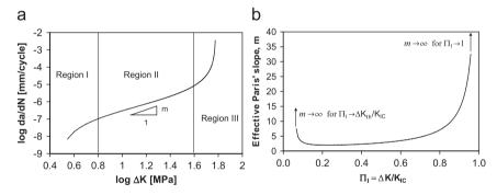
**Fig. 1.**  $\Pi_1$ -dependence of the Paris' law parameter m. (a) A typical da/dN curve for steel (R=0,  $K_{IC}=60$  MPa $\sqrt{m}$ ,  $\Delta K_{th}=3$  MPa $\sqrt{m}$ ). (b) Effective Paris' slope m vs.  $\Pi_1=\Delta K/K_{IC}$  computed from (a).
