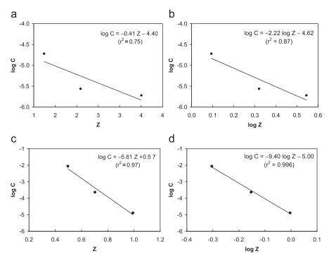
**Fig. 6.** Assessment of incomplete self-similarity in  $\Pi_5$  in concrete (C evaluated using  $\Delta K$  in MPa  $\sqrt{m}$  and da/dN in m/cycle). (a) and (b) High strength concrete (data from Bažant and Shell, 1993 reinterpreted by Spagnoli, 2005). (c) and (d) Normal strength concrete (data from Bažant and Xu, 1991 reinterpreted by Spagnoli, 2005).
