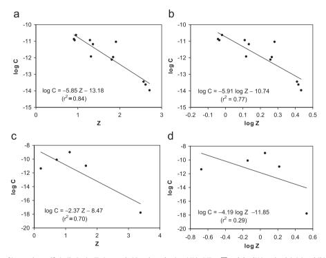
Fig. 5. Assessment of incomplete self-similarity in  $\Pi_5$  in metals (C evaluated using  $\Delta K$  in MPa  $\sqrt{m}$  and da/dN in m/cycle). (a) and (b) 4340 steel (Heiser and Mortimer, 1972). (c) and (d) ASTM steels (Clark and Wessel, 1970).
