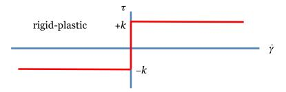
In the limit of vanishing viscosity during flow, the viscoplastic model reduces to the rigid-plastic model. In the limit of vanishing yield stress, the viscoplastic model reduces to the viscous model.
