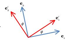
For a given state of stress, its components change when the basis changes. A state of stress  $\sigma$  is a physical fact, and is independent of the choice of the basis. Given a basis, we picture a unit cube with edges coinciding
