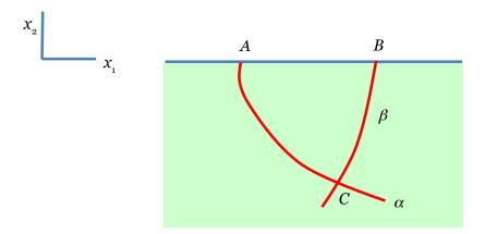
**Flat, traction-free boundary**. A flat, traction-free boundary lies on the  $x_1$ -axis,  $\sigma_{12} = \sigma_{22} = 0$ . If the material beneath flows, it obeys the yield condition:
