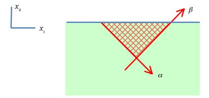
**Compression without friction.** A boundary lies on the  $x_1$ -axis. The boundary satisfies the condition  $\sigma_{12} = 0$ . Thus, the boundary is normal to a principal stress, and the orientation of slip is at 45 degrees from the  $x_1$ -axis. The field of stress and the field of velocity are both homogeneous in the triangle beneath the boundary.
