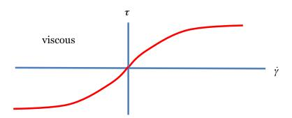
**Viscoplastic flow.** In a viscoplastic flow, the relation between the shearing stress and the rate of shear is not one-to-one. Let k be the yield stress. When the shearing stress is within the yield stress,  $|\tau| < k$ , the fluid is rigid,  $\dot{\gamma} = 0$ . When the shearing stress exceeds the yield stress,  $|\tau| > k$ , the fluid flows. The fluid may flow in a complicated way. It may shear-thin, strain-harden, or be thixotropic.
