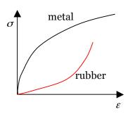
**Fit a stress-strain curve to an expression**. For a **metal** undergoing large, plastic deformation, the stress-strain curve (without unloading) is often fit to a power law:
